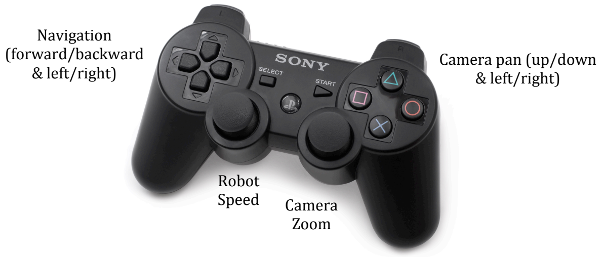
Figure 1: Gaming controller ground control interface
